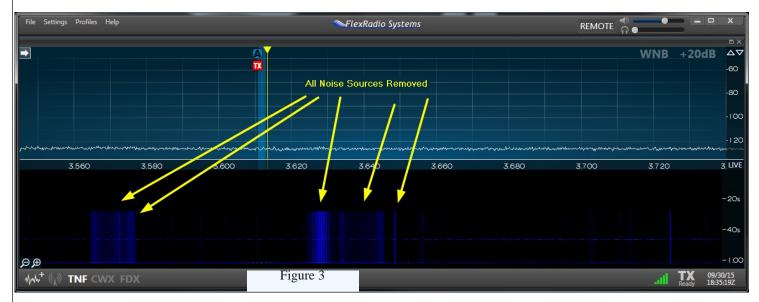
Figure 3 shows what can be done when all significant sources of noise have been removed from the 80 meter band. Remember the time? Its 18:35 UTC or 2:35 pm local time and 80 meters is dead at that time!
