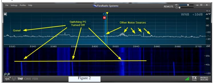
In *Figure 2* the wall wart has been unplugged after about thirty seconds have elapsed on the display. The instantaneous panadapter shows that the wall wart 'signature' has disappeared while the waterfall shows
